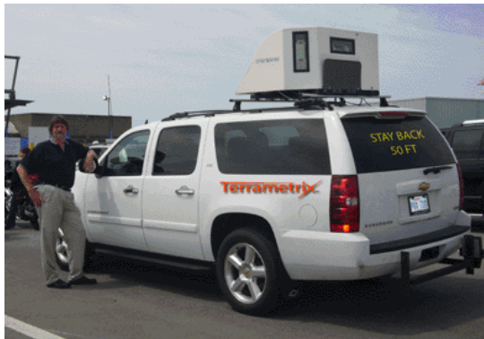
Scan vehicle has 4 scanners, up, down, left and right with video forward and back.
